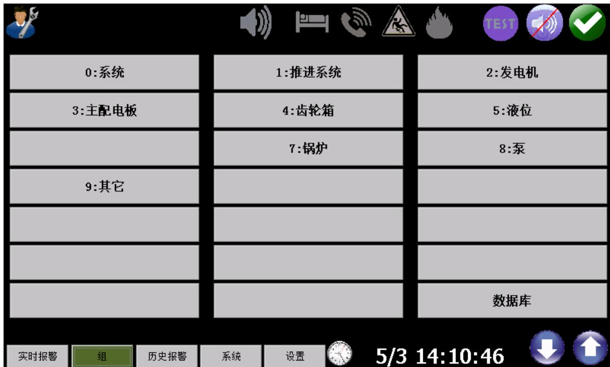
点击组按钮可以进入相应的组查看测量点的信息如下: Click on the button can enter the corresponding group check measurement point information is as follows:
